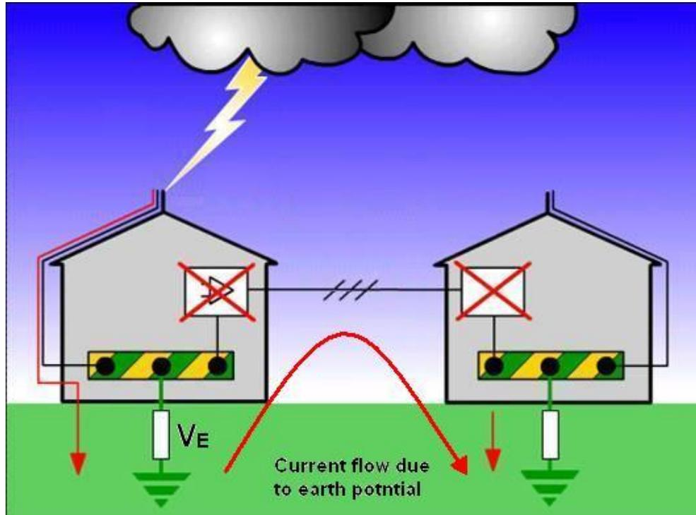
Figure 5. Resistive coupling
