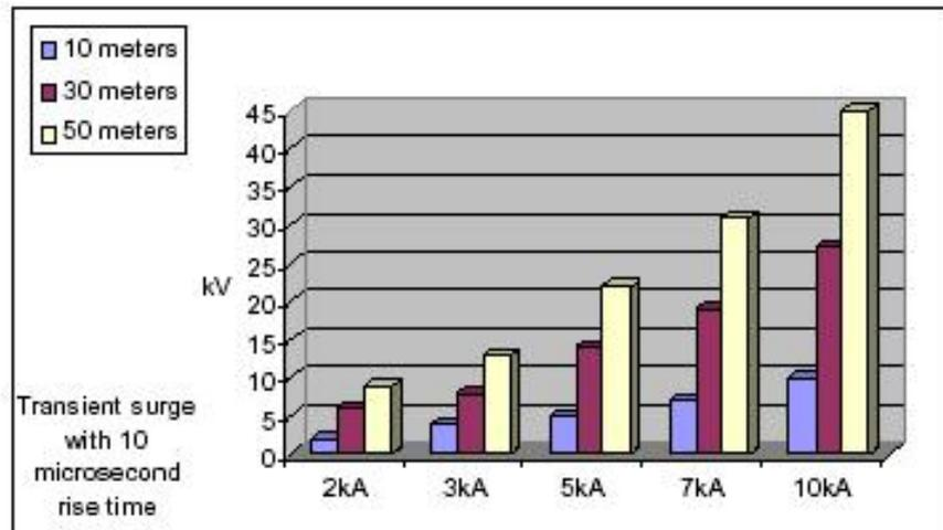
Figure 6. Lightning current on different length of wire
