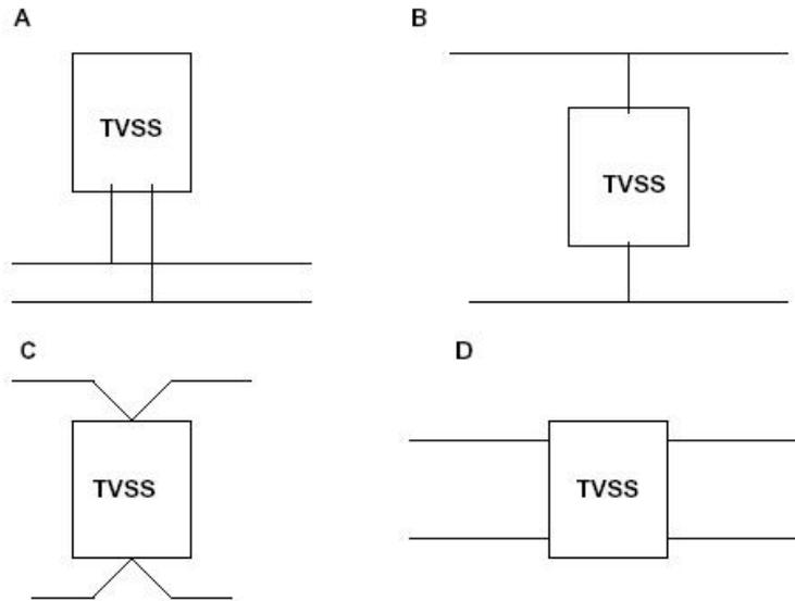
In diagrams A & B the devices are far less effective at reducing a transient surges, because of the impedance of the connecting wires. In tests we found a 700V drop in 500mm x 6mm<sup>2</sup> wire for a 6kV x 3.3kA transient, which will be made far worse by the addition of a TVSS isolating mcb.
