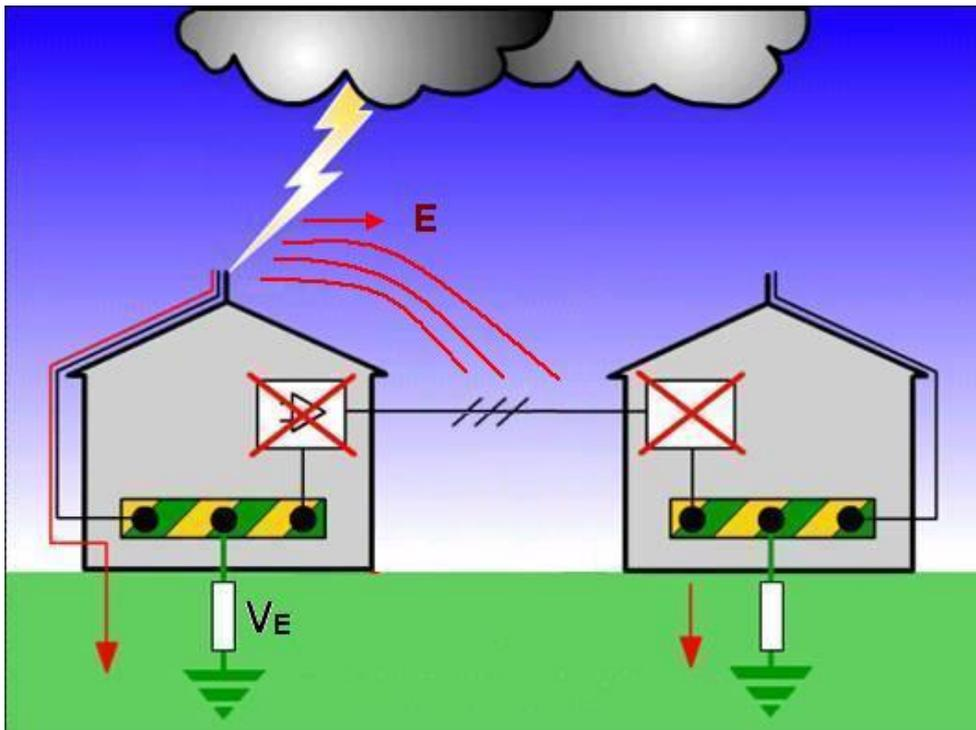
Figure 4. Capacitive coupling
